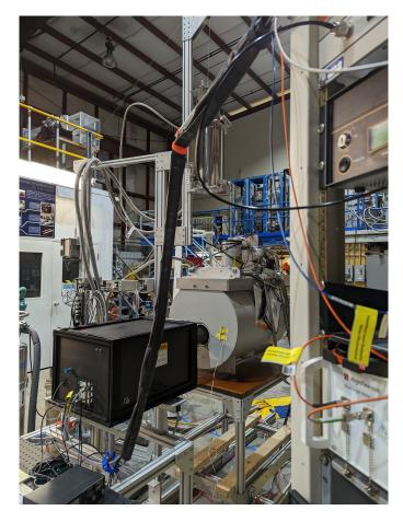
**Figure 3:** Photo of the polarization stand. The laser enclosure in black extends into the warm-bore of the superconducting solenoid to hold the pumping cell in the uniform field region.
