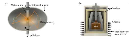
**Figure 1:** (a) Floating Zone system: In the FZ method, the whole of the material rods are sequentially crystallized from the bottom by cooling the melted part through moving the mirrors upward slowly. (b) Czochralski system: The Cz method grows large bulk crystals by pulling up the melted raw material in the crucible under a temperature gradient.
