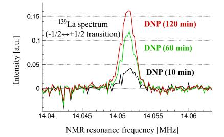
**Figure 3:** Enhancement of the <sup>139</sup>La NMR peak ( $-1/2 \leftrightarrow +1/2$  transition) at 1.3 K and 2.3 T using the sample of 0.01 mol% Nd concentration. The NMR peaks are shown at elapsed times of 10 min (black), 60 min (green), and 120 min (red) after the microwave irradiation.
