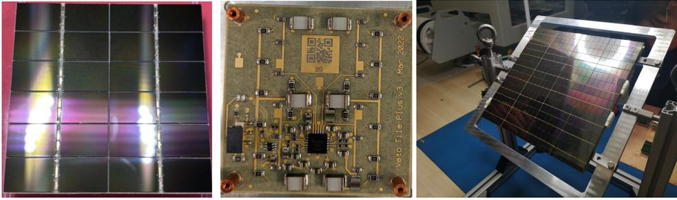
**Figure 1:** Left: Front and back side of a veto tile. Right: a vPDU
