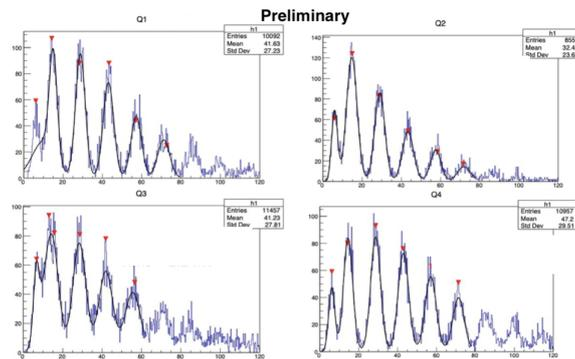
**Figure 5:** Amplitude spectra for each quadrant of the vPDU.
