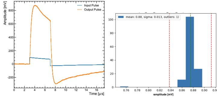
**Figure 3:** Left: charge injection pulse in blue and output pulse in orange. Right: distribution of pulse amplitude
