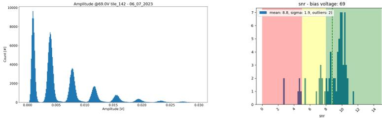
**Figure 4:** Single tile amplitude spectra of a single tile and SNR distribution from pre-production tile testing.
