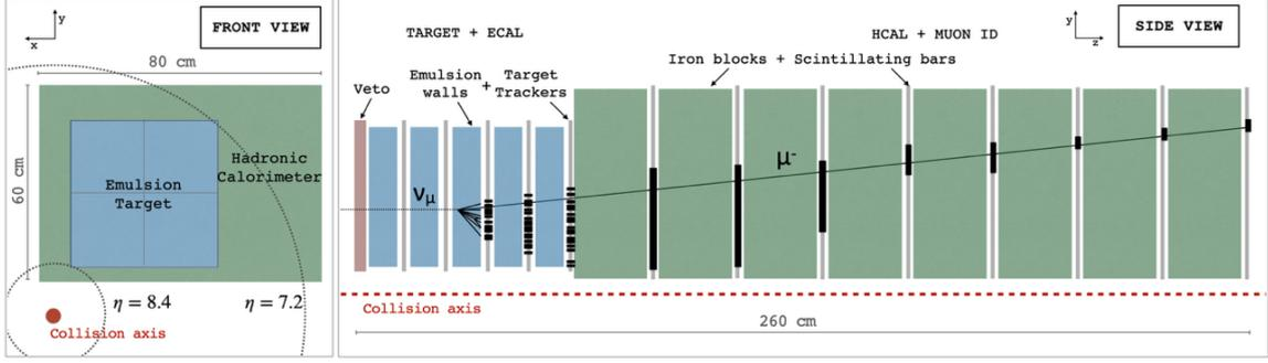
**Figure 1:** Schematic layout of the SND@LHC detector front view (left) and side view (right).
