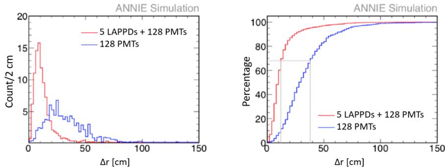
**Figure 3:** ANNIE simulation for, on the left side, the vertex and on the right side, the direction resolution for reconstructed events with only PMTs (blue) and PMTs and 5 LAPPDs (red). [3]
