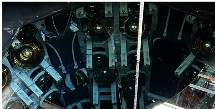
**Figure 5:** Inside view of the ANNIE tank. All deployed LAPPDs as well as some of the mounted PMTs can be seen.
