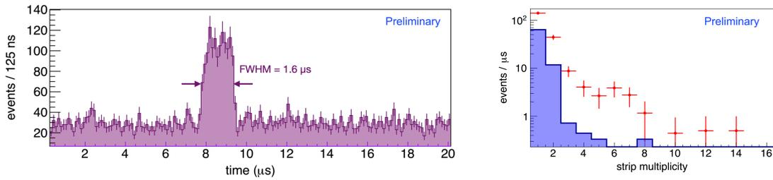
**Figure 4:** The left plot shows the event time distribution from the LAPPD. Shown is the time from the beam acquisition window start to the event timestamp. An excess of events with a FWHM of  $1.6 \mu\text{s}$  can be seen, which matches the BNB beam window. The right plot shows the strip multiplicity with the rate normalized to events/ $\mu\text{s}$  for on-beam data (red) and off-beam data (blue).
