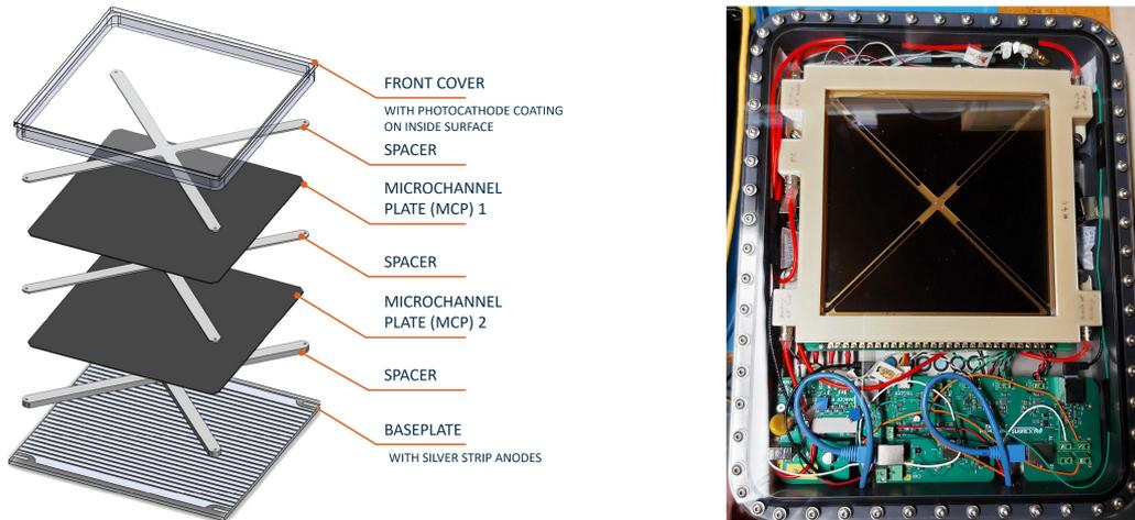
**Figure 2:** The left picture shows the LAPPD schematic setup. From the top: a borosilicate glass + cathode cover window, two levels of spacers and MCPs and a baseplate with strip line anodes at the bottom [2]. The right picture shows the complete LAPPD package as used in ANNIE. It contains the LAPPD with its mounted ADCs as well as a slow control board for sensor readout and voltage control.
