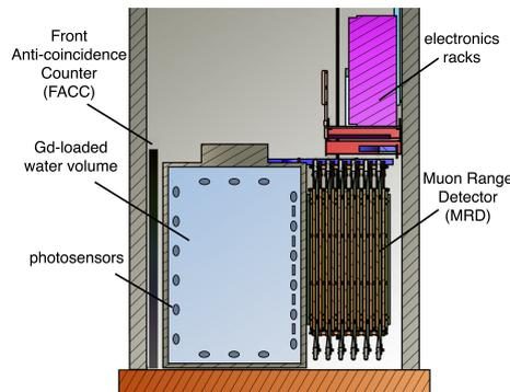
**Figure 1:** Schematic representation of the ANNIE detector setup. [1]
