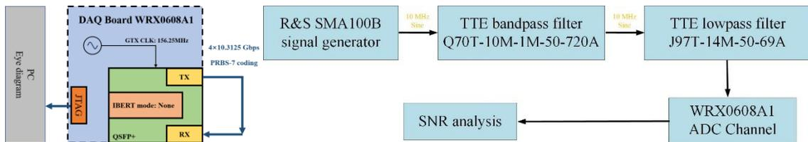
**Figure 2.** The test setup of QSFP+ high speed lane signal integrity (left) and the test setup of ADC's ENOB (right).
