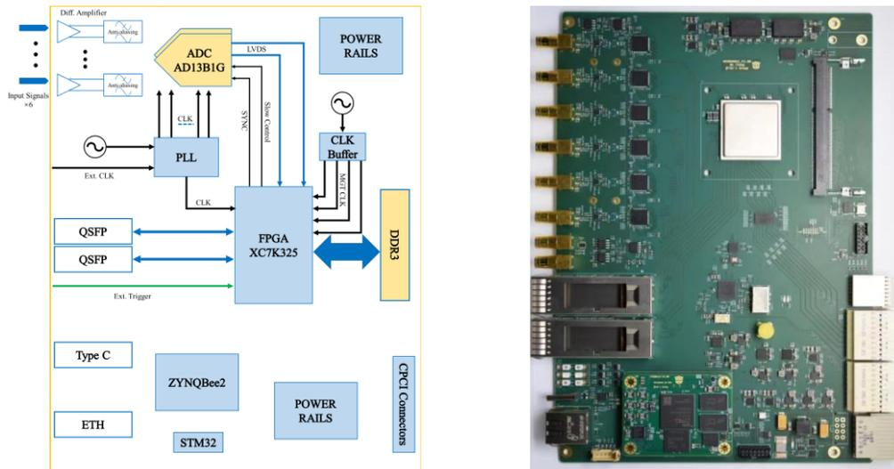
**Figure 1.** WRX0608A1 waveform digital system architecture diagram (left) and PCB physical photo (right).
