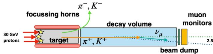
**Figure 2:** Schematic view of the proton beam interacting in the T2K target.
