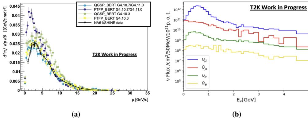
**Figure 6:** (a) Pion yields from G4JNUBEAM simulations (markers) and NA61/SHINE data (solid line) for the last 18 cm downstream of the target in the 20-40 mrad angular range and (b) G4JNUBEAM neutrino fluxes at ND280 (for a horn current of 320 kA).
