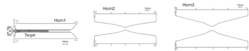
**Figure 3:** Cross section of the three magnetic horns showing the graphite target inside the first horn. Adapted from [1].
