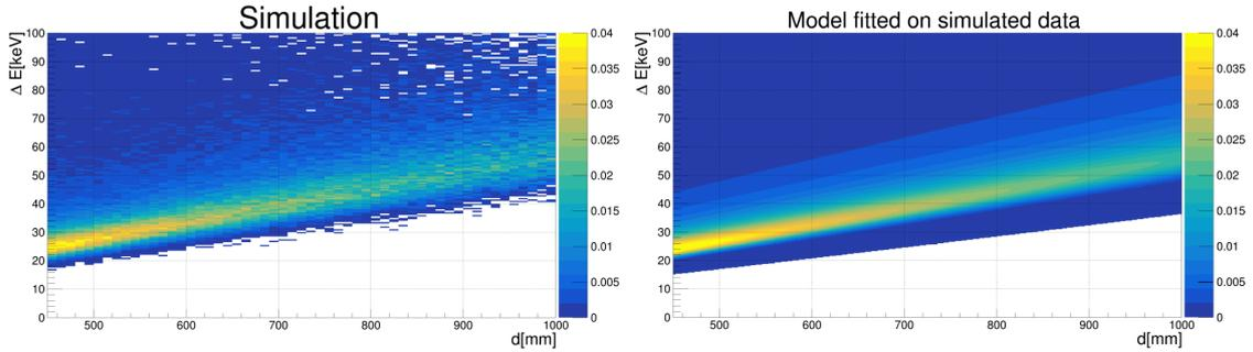
**Figure 2:** A comparison of the distribution of energy losses of electrons obtained from a simulation of the calibration measurement and theoretical model fitted on the data (not normalised).
