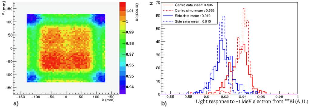
**Figure 3:** a) Simulation of the front face of a scintillator block, showing the difference in light collection as a function of the impact point of the incident electron [4]. b) Difference in the scintillator response to  $^{207}\text{Bi}$  electrons (976, 1048 and 1060 keV) impacting in different regions.
