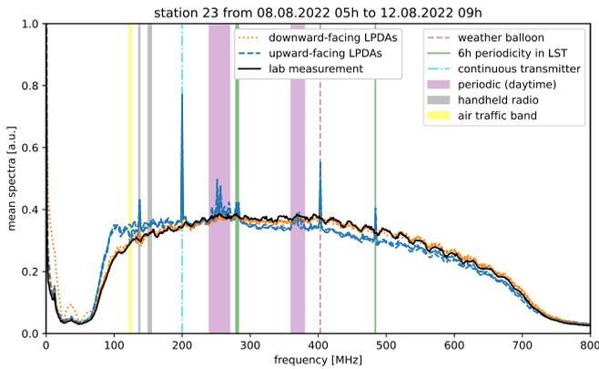
**Figure 4:** Average frequency spectra observed in the upward- and downward-facing LPDAs. A lab measurement of average noise spectra of the DAQ system alone is added for comparison. The spectra are normalised with respect to each other in the 500–650 MHz region. Known narrowband and broadband backgrounds are indicated in the legend.
