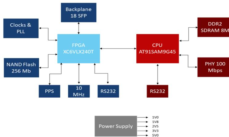
**Figure 6:** Diagram of the main blocks that form the so-called White Rabbit Switch.
