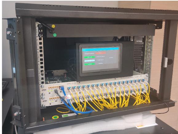
**Figure 7:** System test for the functional test of the switching core boards. The automatization of the production is of crucial importance for increasing the reliability of the boards to be used in the experiment.
