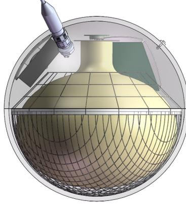
**Figure 2:** Optical module design schematic. A 20-inch PMT encapsulated inside a 23-inch glass sphere.
