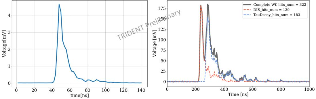
**Figure 3:** The left figure shows the PMT waveform template obtained from laboratory measurements. The right figure is a typical double pulse waveform, where the red and blue colors represent the photons originating from the DIS vertex and the tau decay vertex, respectively.
