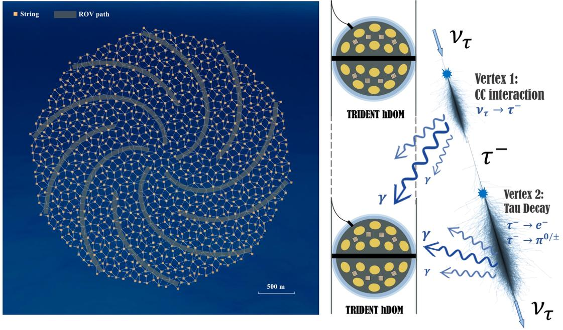
**Figure 1:** The TRIDENT Penrose geometry and the tau neutrino interaction process in the detector
