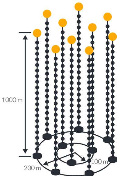
**Figure 1:** A sketch of a cluster of P-ONE mooring lines. The full scale detector is planned to consist of seven clusters. Figure adapted from Ref. [1]
