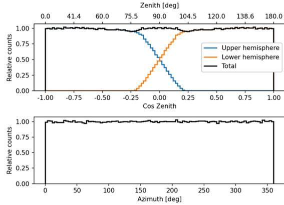
(b) Geant4 isotropy simulation results
