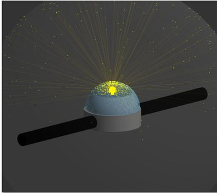
(a) Geant4 isotropy simulation setup
