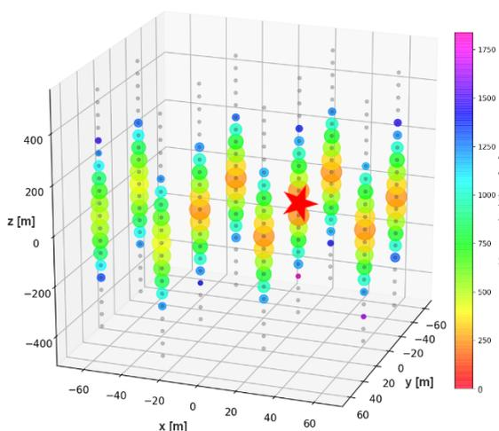
**Figure 7:** Simulation of a P-CAL flash propagating through a P-ONE cluster. The red star at the origin represents the P-CAL. The coloured dots represent other modules detecting light with arrival time and intensity shown as colour and size respectively.
