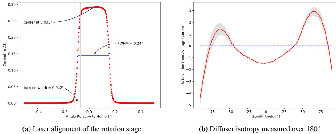
**Figure 8:** (a) shows the preliminary result zenith alignment sweep. This indicates a resolution of  $0.24^\circ$  and that the zero angle needs to be readjusted to  $0.033^\circ$ . (b) shows a preliminary isotropy measurement of a teflon diffuser. The red line is an average over 12 azimuthal measurements. This first measurement shows a maximum 4% deviation from the average photodiode current over the entire sweep range.
