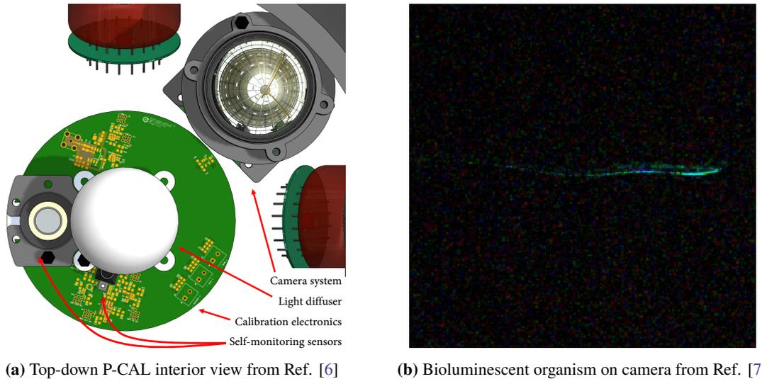
**Figure 4:** (a) shows an interior view of the P-CAL. The self-monitoring photodiode and SiPM are positioned to the left and bottom-left of the diffuser sphere respectively. The camera is mounted in the top right corner of the image. (b) is a 60 s exposure image of a bioluminescent organism taken by the a camera in the STRAW-b pathfinder [7].
