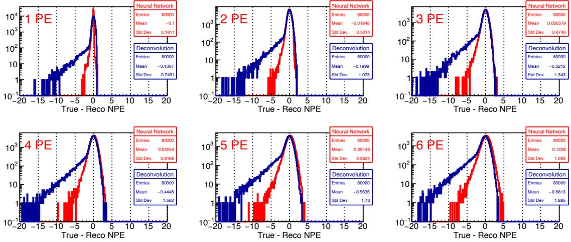
**Figure 8:** Waveform reconstruction results based on training fake waveforms.
