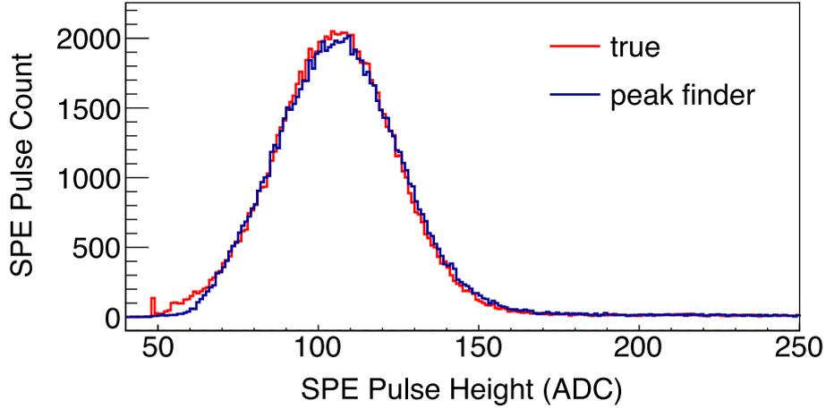
**Figure 4:** Distribution of the pulse height of the SPE found by a pulse finder. At the lower end one can see a deficit between the distribution of the true pulse height and that from the pulse finder. This is due to the small pulses missed by the pulse finder.
