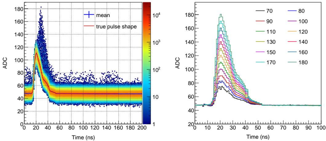
**Figure 5:** Left: An averaging of SPE pulses of similar heights is performed in order to remove the influence of electronic noise. Right: Examples of averaged SPE pulses for some selected pulse heights.
