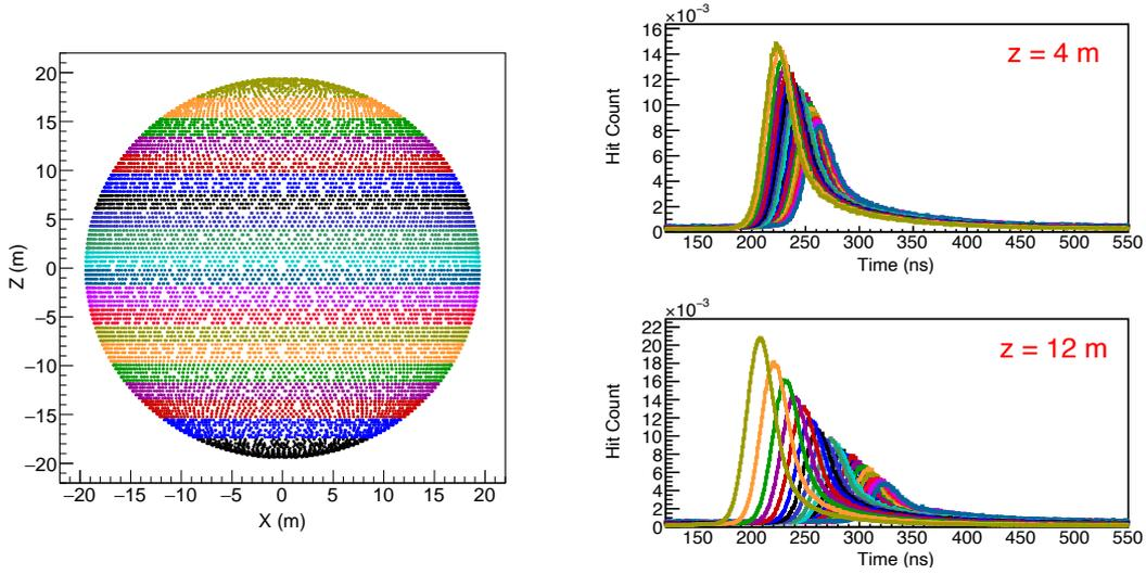
**Figure 6:** Left: PMTs are divided into different groups based on their zenith angle represented by different colors. Right: Example timing PDFs for different source  $z$  positions along the central axis of the detector and groups of PMTs.
