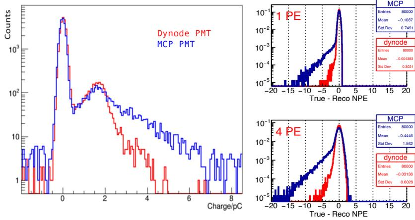
**Figure 2:** Left: “Long tail” observed in the single PE charge distribution of MCP PMTs. The figure is adapted from Reference [2]. Right: the “long tail” gets passed onto the output of a deconvolution-based waveform reconstruction.
