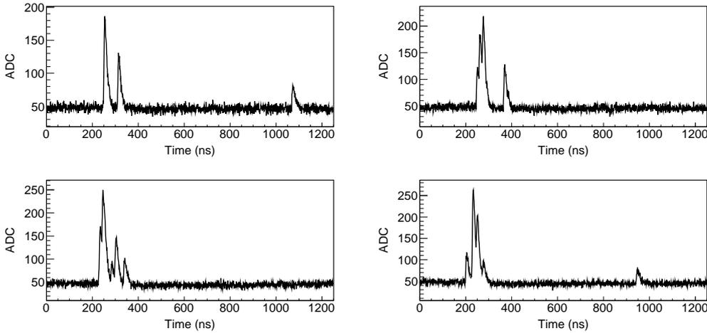
**Figure 7:** Examples of fake waveforms with 4 (top) and 8 (bottom) photoelectrons.
