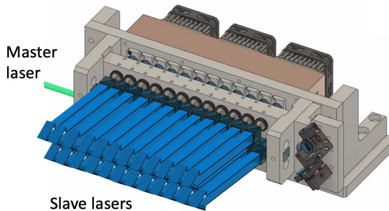
**Figure 1:** A beam splitter device for multiple FP-LDs to produce laser power up to 2W, with controlled wavelength via injection-locking technique.
