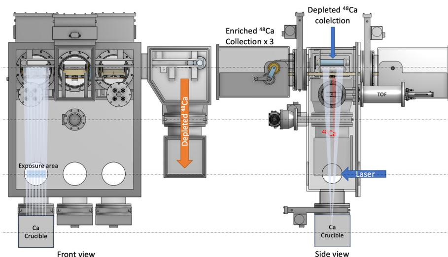
**Figure 2:** Schematic diagram of the irradiation unit for a large-scale production system (2 mol/year). (Left) Front view, (Right) Side view
