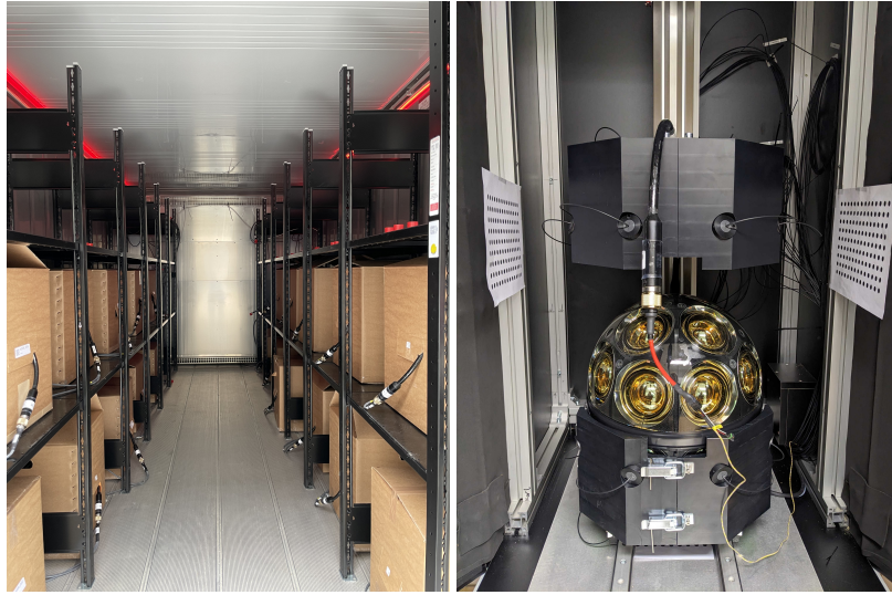
Figure 4: FAT facility at DESY. Left: DFL loaded with 24 mDOMs inside their boxes. Right: Optical FAT setup, with 24 optical fibers routed through a support structure.
