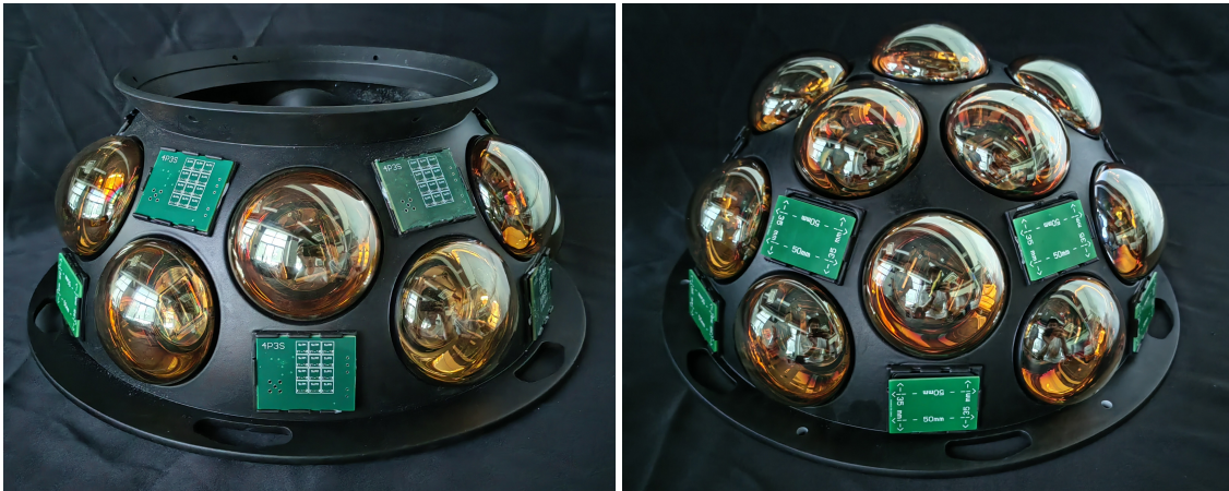
Figure 3: The 3D-printed shell to house the photo-sensor brackets. The left and right images show the upper and lower hemispheres, respectively.
