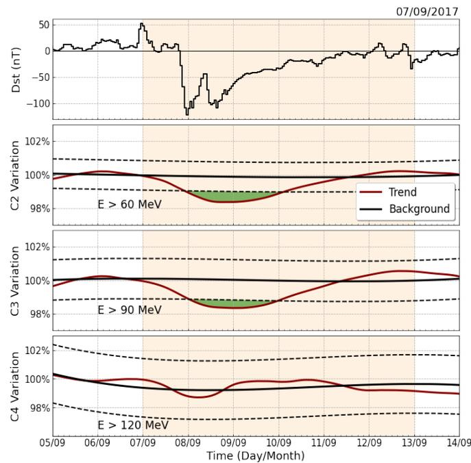
**Figure 2:** GS of September 7th 2017. The top panel shows the Dst index. The lower three panels show SNT's charged particle channels percentage variations.
