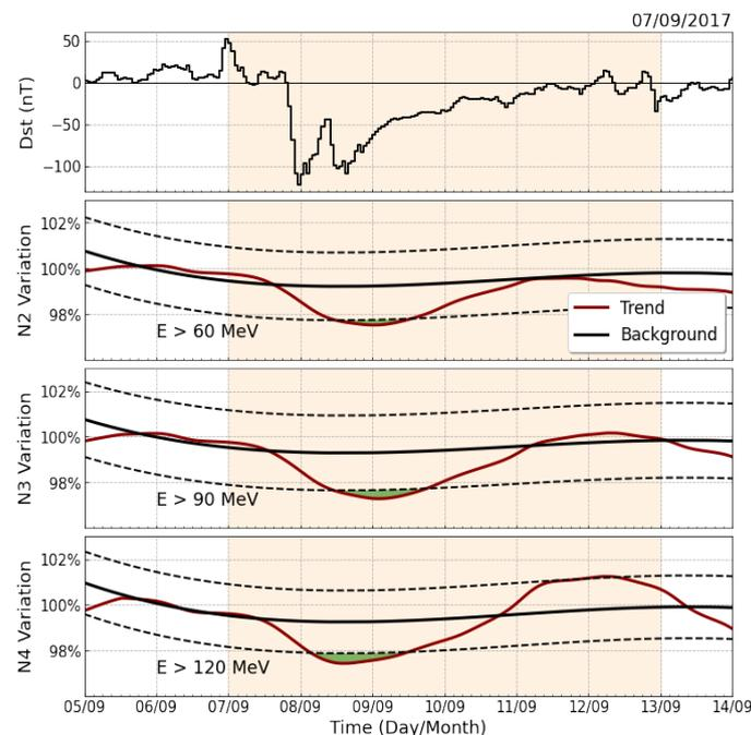
**Figure 1:** GS of September 7th 2017. The top panel shows the Dst index. The lower three panels show SNT's neutral particle channels percentage variations.
