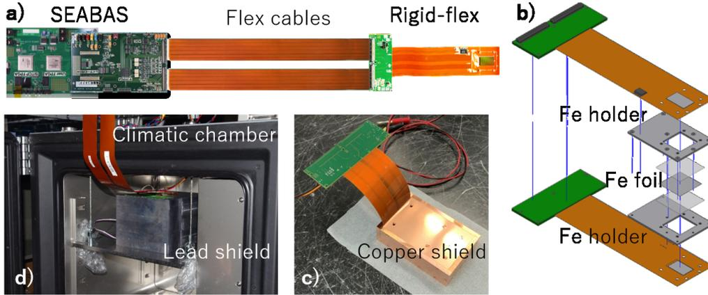
**Figure 2:** Readout of XRPIX using rigid-flexible circuit board. a) shows a readout unit of a XRPIX7. b) represents schematic drawing of a module composed of two XRPIXs. c) and d) are pictures of copper and lead shield, respectively.
