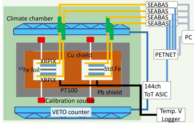
**Figure 1:** Schematic drawing of ISAI detector.
