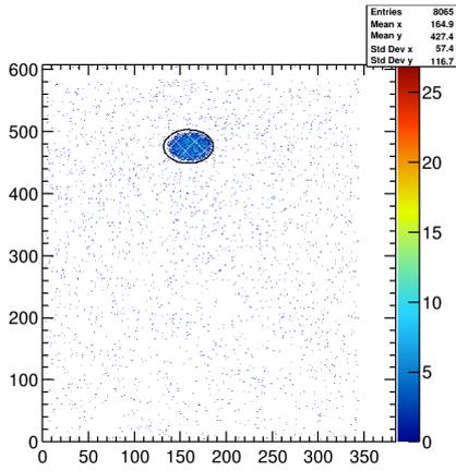
**Figure 3:** Demonstrated hit map distribution irradiated by  $^{241}\text{Am}$  source through pin hole in the shield. The black line and blue line show the energy distribution of pixels inside and outside of pin-hole, respectively. The red lines show signal boundary defined by the FWHM 2.8 keV at 13.9 keV around 14.4 keV.
