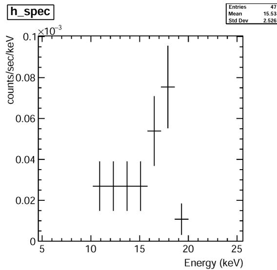
**Figure 6:** Raw background distribution of ISAI detector module using a standard Fe foil.
