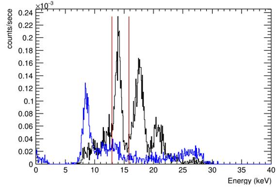
**Figure 4:** Demonstrated energy distribution irradiated by  $^{241}\text{Am}$  source in Fig.3. The black line and blue line show the energy distribution of pixels inside and outside of pin-hole, respectively. The red lines show signal boundary defined by the FWHM 2.8 keV at 13.9 keV around 14.4 keV.
