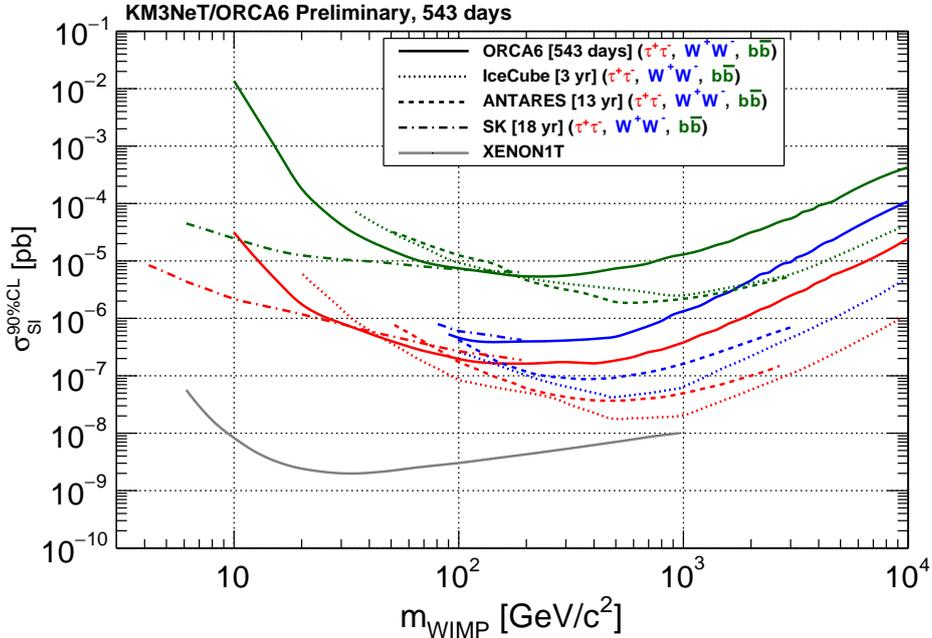
**Figure 3:** The 90% CL upper limits on the spin-independent WIMP-nucleon cross section as a function of the WIMP mass for each of the three annihilation channels. The full lines show the results obtained in this analysis, whereas the other lines show the upper limits obtained by IceCube [8], ANTARES [9], Super-Kamiokande [10] and XENON1T [12] (shown as a full line).
