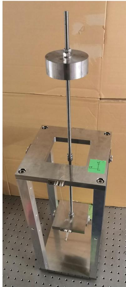
**Figure 4:** Picture of the benchtop prototype. The RL frame is suspended with four wires. The counterweight is attached to the vertical rod.
