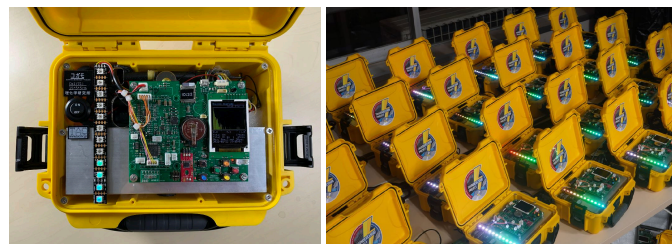
Figure 2: (left) Photo of a compact gamma-ray monitor (CoGaMo) used by the citizen science "Thundercloud Project." (right) Multiple Cogamos with turning on the LED lights on the detector boxes.
