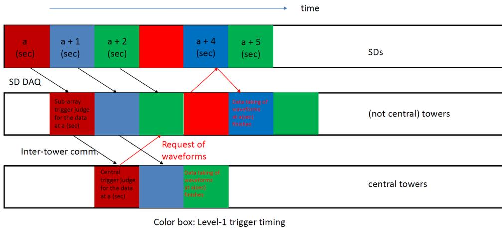
**Figure 2:** Time sequence of the data acquisition including inter-tower triggers. Boxes with different colors denote Level-1 trigger times collected at different seconds.
