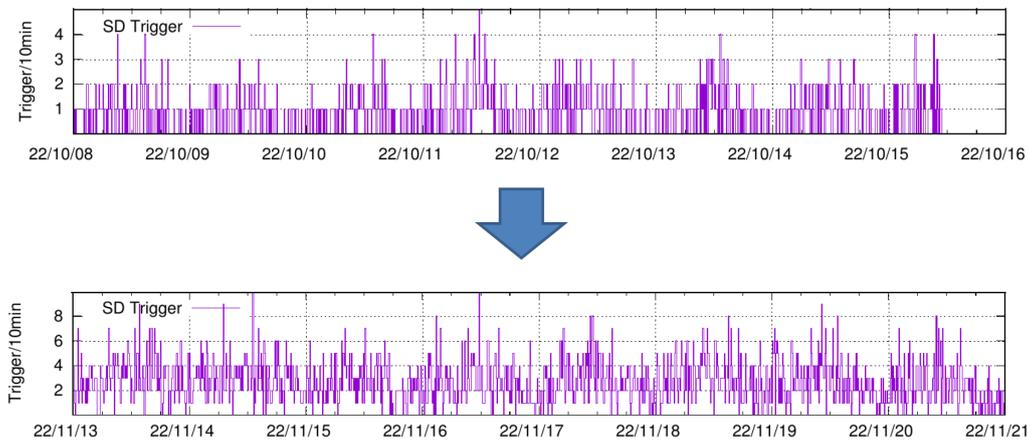
**Figure 3:** Updates of the Level-2 trigger rates at the north central tower before and after implementing inter-tower triggers.
