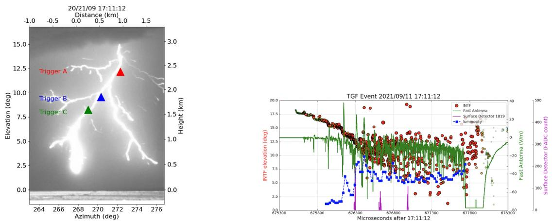
**Figure 2:** *Left:* This figure shows the elevation vs. azimuth for the whole flash in a frame of the camera. The red, green, and blue triangles are the sources of the TGF for triggers A, B, and C consecutively. *Right:* This figure shows the TASD waveforms for one of the SDs in magenta, the average luminosity in dark blue, the electric-field waveform in green, the INTF elevation in red circles. The flash observed from initiation until the first return stroke within 3 ms duration.
