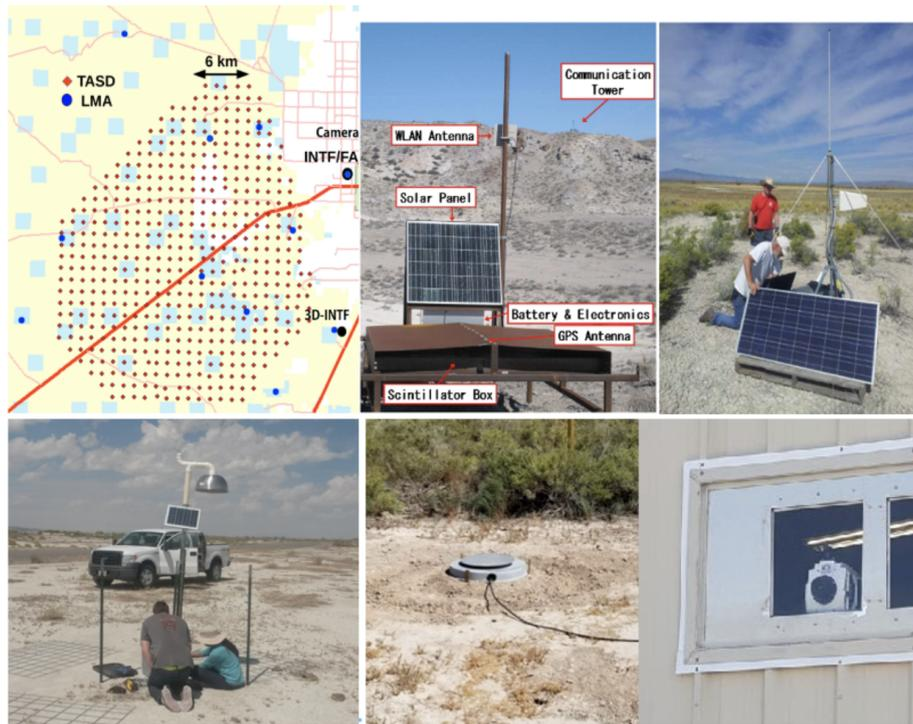
**Figure 1:** From left to right, the Telescope Array and lightning instruments detectors map, the surface detector, the LMA station, the slow antenna station, the interferometer, and the high-speed-video camera.
