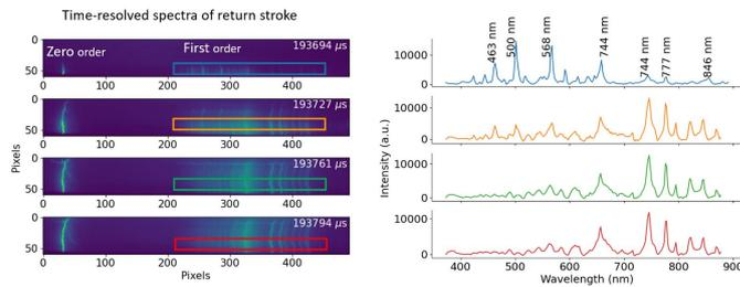
**Figure 3:** *Left:* The Phantom high-speed video camera v2012 and the v711. *Middle:* A series of the return stroke spectral images which were recorded by our spectroscopic system, at 29,990 frames per second by the Phantom V711. *Right:* From each image in the middle figure, a section of  $8 \times 230$  pixels was selected of the first order of the dispersion to get the time-resolved spectra of the return strokes.
