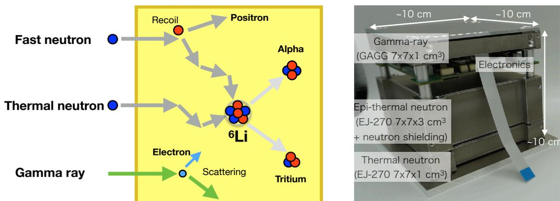
**Figure 2:** (Left) Structure of 1 unit with a scintillator and SiPMs. (Right) Structure of the MoMoTarO detector.
