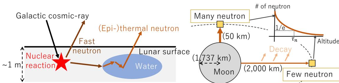
**Figure 1:** (Left) Thermal and epi-thermal neutrons leaking from the lunar surface. (Right) Neutron lifetime measurement using a lunar elliptical orbit.
