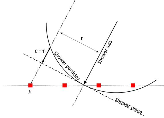
**Figure 2:** Schematic diagram of an air shower and TALE-SDs. The red squares are TALE-SDs, the dashed line is the shower plane and the black curve shows the positions of the shower particles.  $\tau$  is the delay in particle arrival time from the shower plane,  $c$  is the light speed,  $r$  is the distance from the shower axis to the SD and  $\rho$  is the particle number density recorded by the SD.
