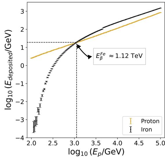
**Figure 4:** Energy lost by muons at a 3m height Water Cherenkov Detector (WCD) as a function of primary energy. This is for an observation level of 4800 masl. The energy lost is a proxy to signal generated in the WCD.
