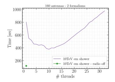
**Figure 5:** The parallelized radio module running on an electron induced air shower processing a detector array of 160 antennas. 2 formalism, namely CoREAS and ZHS are activated and use 160 antennas each. The performance peaks at 10 worker threads, beyond which the performance degradates.
