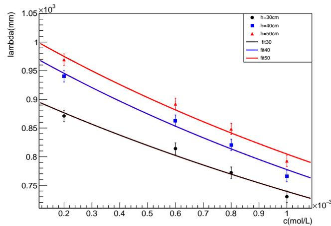
**Figure 6:** The effective attenuation time and absorption coefficient obtained by fitting three sets of data with the height of 30 cm, 40 cm, and 50 cm.
