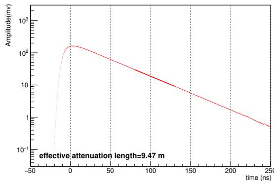
**Figure 5:** The effective attenuation length obtained by the device under 532 nm laser.
