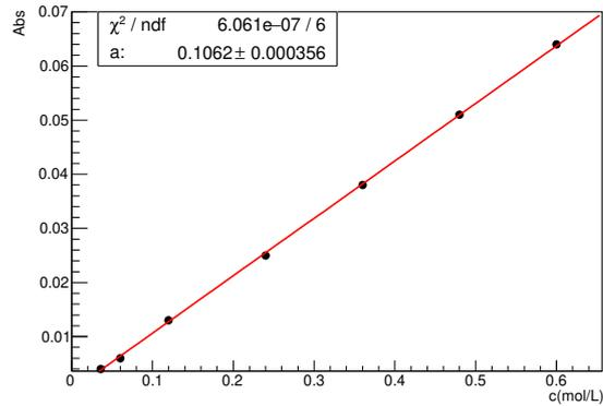
**Figure 4:** Absorption coefficient of copper sulfate solution at 532nm.
