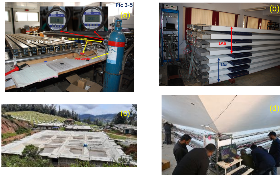
Figure 5: (a) Test bench for PRC vacuum creation and gas filling, (b) testing of PRC performances, (c) 16 modules of the new muon telescope, and (d) operation of the first module of the new muon telescope.
