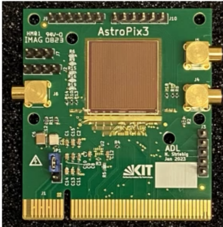
(a) One 2 \times 2 \text{ cm}^2 AstroPix_v3 chip mounted to a board for bench testing
