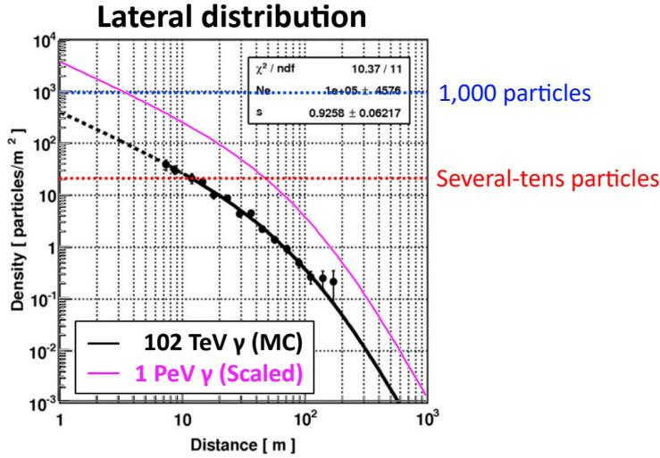
**Figure 1:** Lateral distribution of showers produced by 102 TeV and 1 PeV gamma rays[1]. The black dots are the results of Monte Carlo simulations for 102 TeV gamma rays. The solid black line is the NKG function fitted to the data for the distance over 10 m, and the dashed black line is the extrapolation of the fitted NKG function for the distance within 10 m. The solid magenta line representing the 1 PeV gamma ray is the black dashed line multiplied by 10 on the vertical axis.
