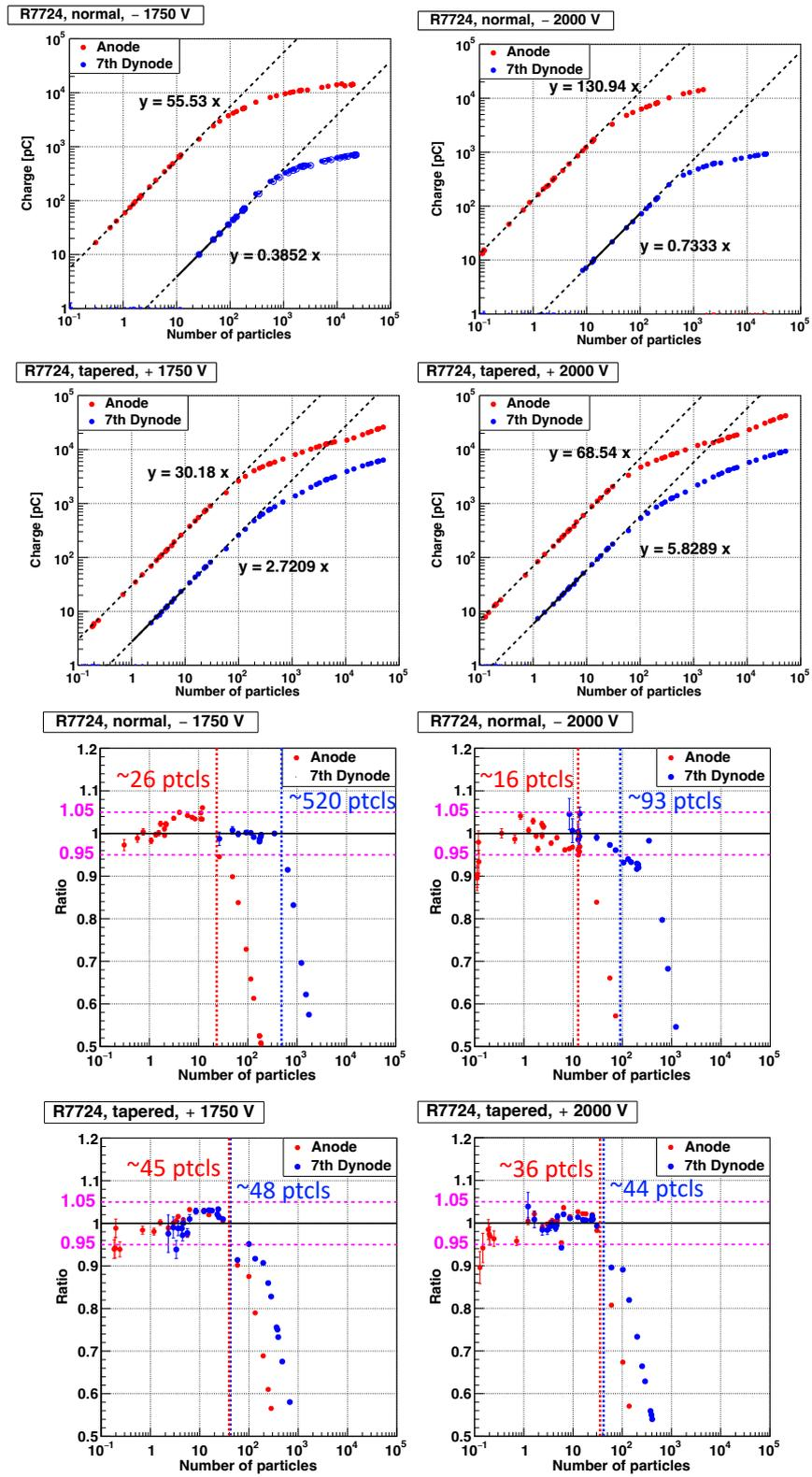
Figure 4: Measurement results of the dynamic range of 2-inch PMT, R7724.
