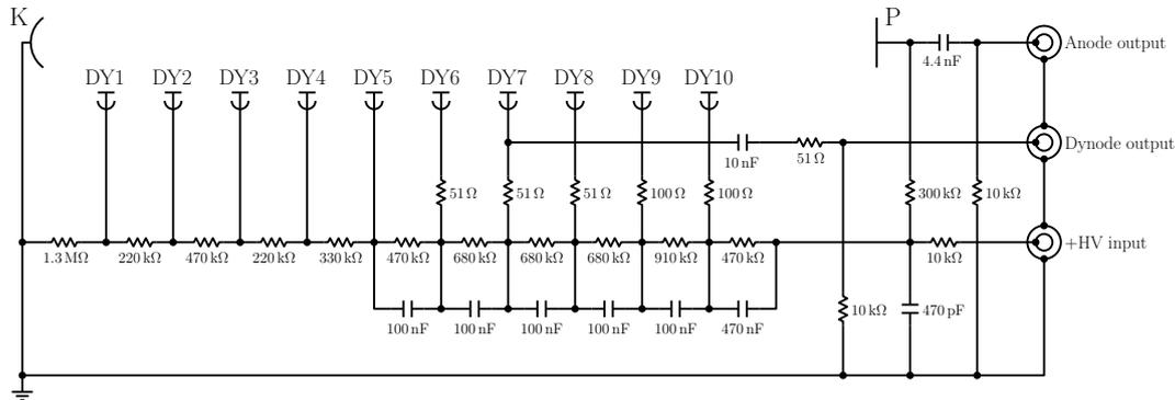
Figure 3: Tapered divider
