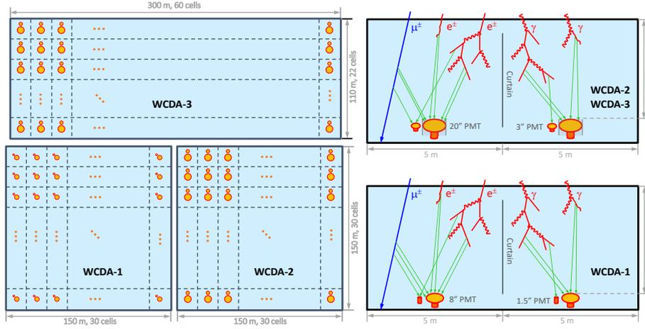
**Figure 1:** LHAASO-WCDA layout and schematic diagram of the interior layout of the detector unit.
