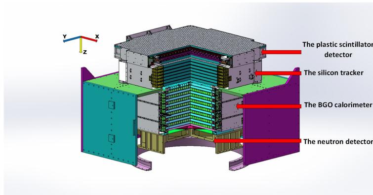
**Figure 1:** Schematic view of the DAMPE detector[1].
