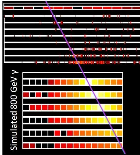
**Figure 6:** A simulated 800-GeV gamma-ray event incident on the CALET calorimeter. Energy losses in each component (CHD, IMC and TASC from the top) are color-coded and a line shows the incident gamma-ray position and direction.
