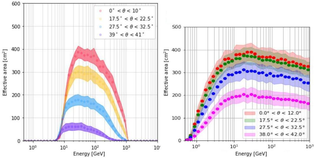
**Figure 7:** Effective area of CALET/CAL for gamma-rays with the standard analysis (for HE triggers, left) and with the improved analysis (right) plotted against gamma-ray energies and some ranges in zenith angles. One can see significant increase of effective area above 100 GeV [13].
