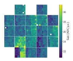
**Figure 3:** Map of the ASTRI-Horn SiPMs gains derived from pulse-height distribution spectra obtained using the internal camera calibration system.
