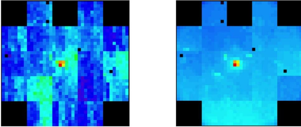
**Figure 7:** Effect of the FF correction to the variance data with the telescope pointed to a bright star. Thanks to the application of the FF parameters, it is possible to see that there are 3 bright spots that do not match any stars in the field of view: these are the so-called *ghosts*, caused by mirror misalignment. The black dots are dead pixels, while one of the PDMs was not working.
