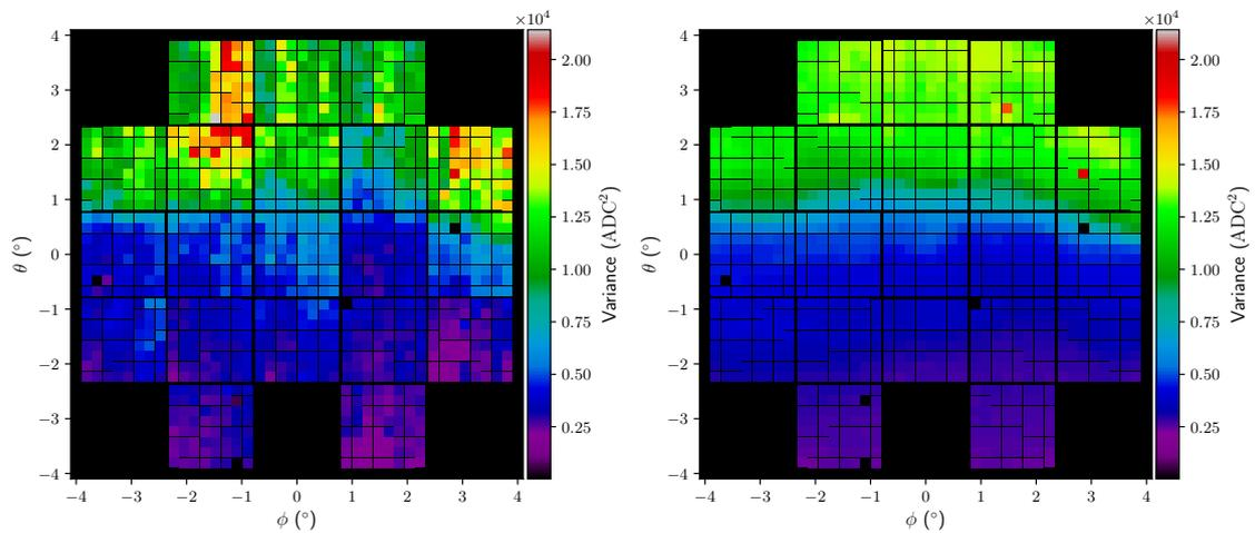
**Figure 6:** Effect of the FF correction to the variance data with the telescope pointed to the South-East crater of the Etna volcano mountain. The black dots are dead pixels, while one of the PDMs was not working.
