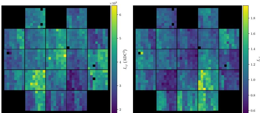
**Figure 3:** The FF image  $I_{i,j}$  (on the left) and the FF correction coefficients  $f_{i,j}$  (on the right) obtained analysing a sample of variance data acquired during the tests of the FF calibration procedure with the experimental set-up shown in Figure 2. The black dots in the FF images correspond to dead pixels. One camera PDM was not working during the tests.
