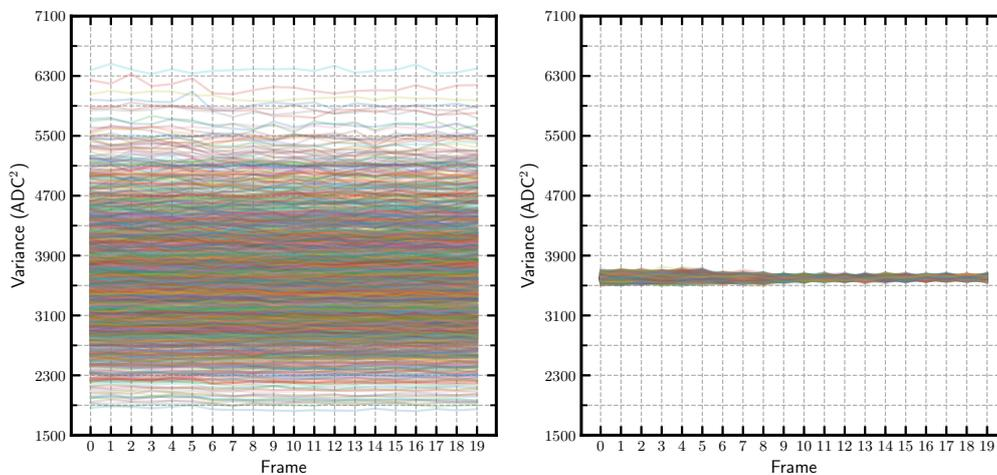
**Figure 4:** On the left, the plot of the 20 chosen frames of the selected run's variance data, without the FF parameters applied; on the right, the same data with the FF correction.
