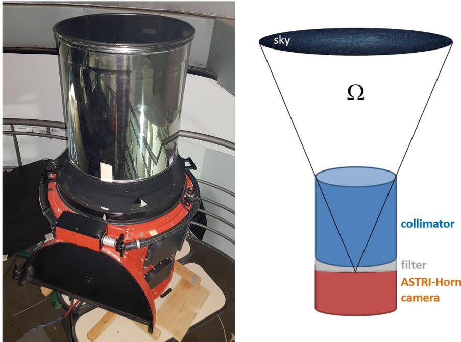
**Figure 2:** The image on the left is a photograph of the set-up used; the image on the right is the set-up model reconstruction, with  $\Omega$  as the angle of open sky visible from the camera, equal to about  $0.012 \text{ sr}$ .
