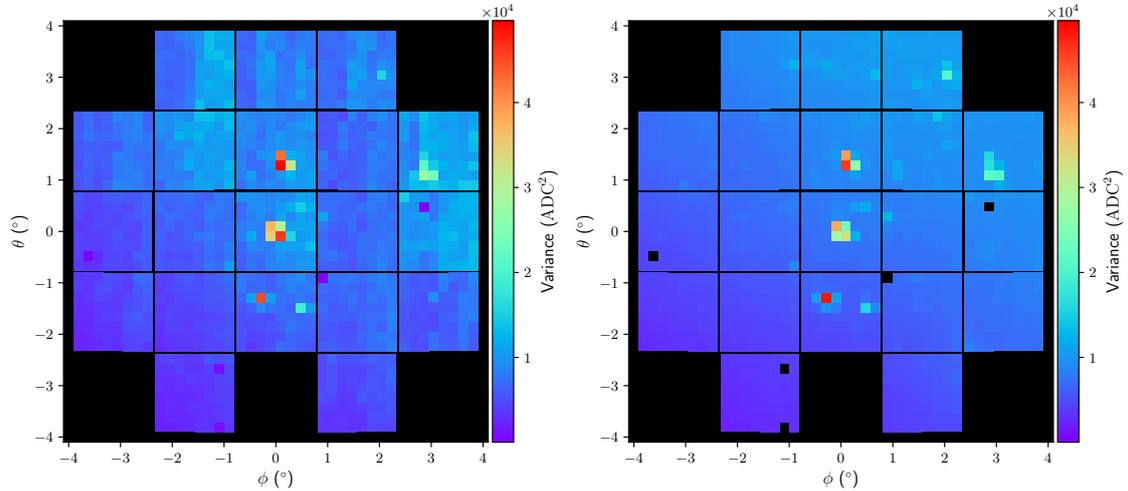
**Figure 5:** Effect of the FF correction to the variance data with the telescope pointed to the Orion's Belt. The black dots are dead pixels, while one of the PDMs was not working.
