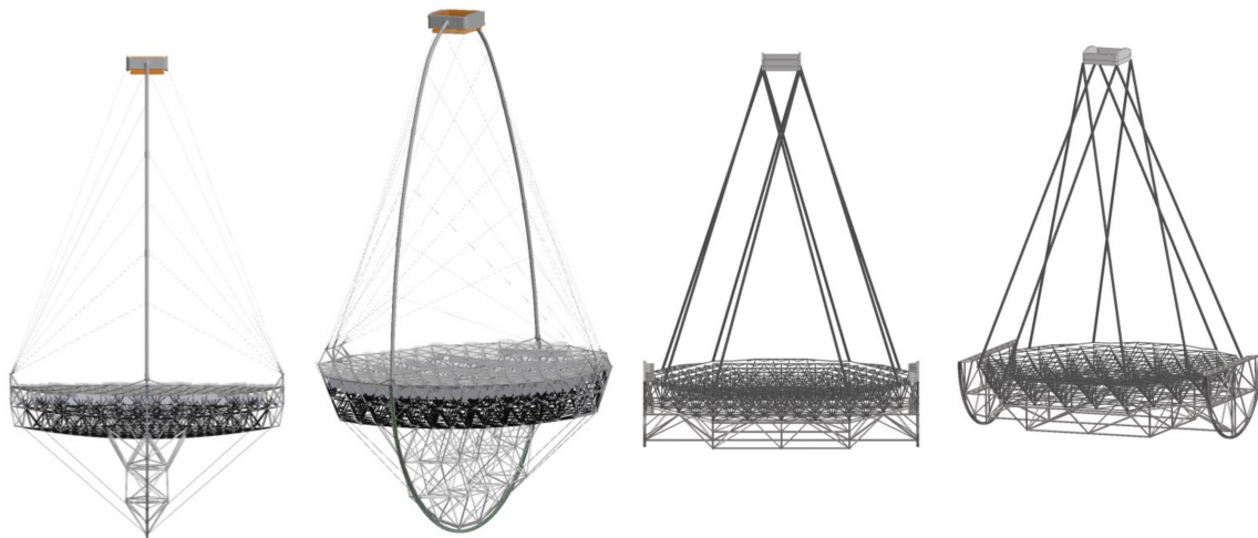
Figure 4: Comparison of elevation structures (left: LST-N, right: concept design for a LST-S structure))
