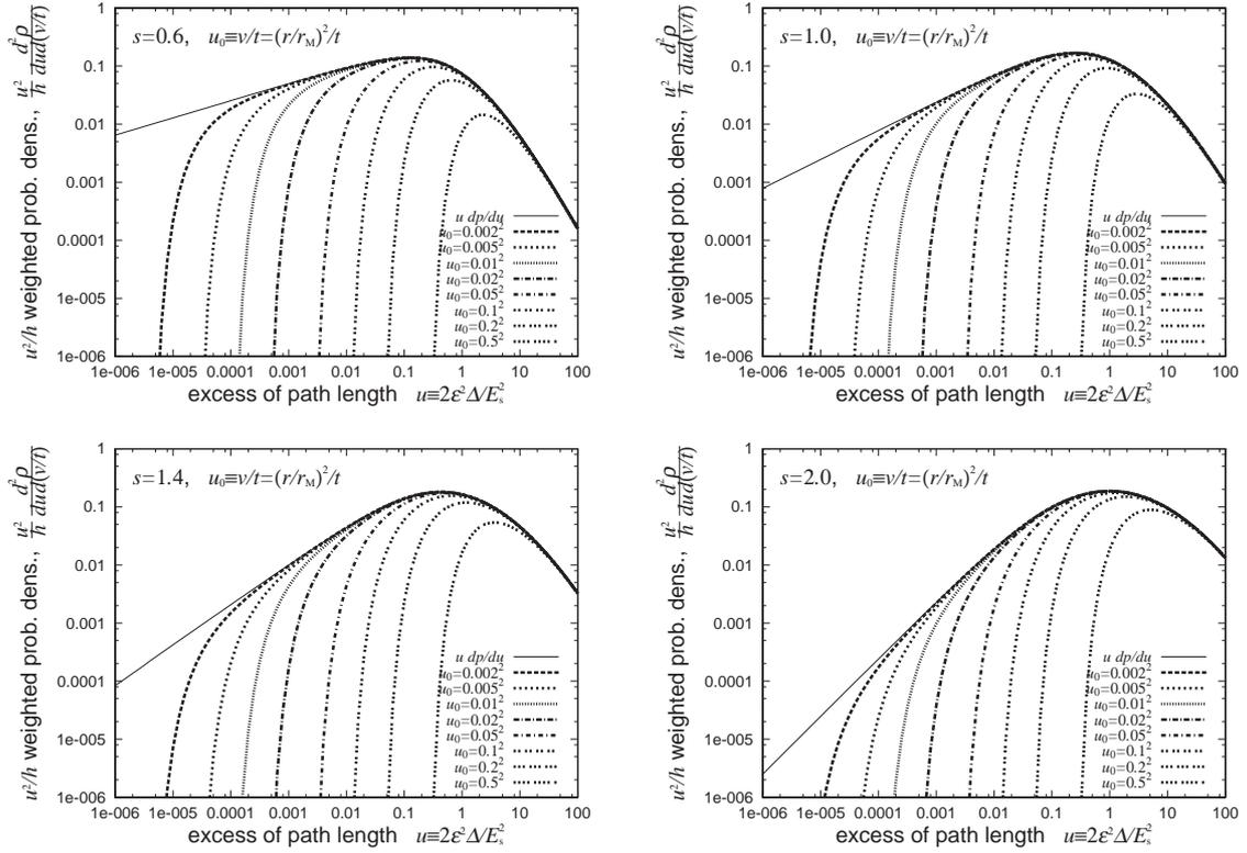
**Figure 1:**  $(u^2/h)$ -weighted probability densities,  $(u^2/h)d^2\rho/du/d(v/t)$ , for excess-path-length of shower electrons at radial distance of  $r$  from the shower axis, for respective ages of  $s$  and parameters of  $u_0 \equiv v/t = (r/r_M)^2/t$  (dot lines). They approach to  $udp/du$  (thin solid line), with the approach of  $r$  to 0. We put  $h = 9$ .
