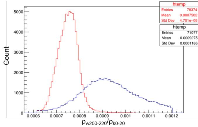
**Figure 3:** The discrimination variable is the ratio between density of the ring from 200 meters to 220 meters to in the WCDA and that from 0 meter to 20 meters in the KM2A. The red one is gamma-ray and the blue is proton.
