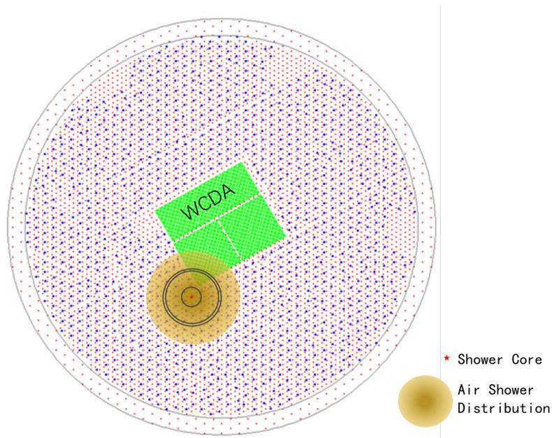
**Figure 1:** Two parts of LHAASO layout are shown above, the red (ED) and blue (MD) dots are KM2A, and the green rectangles are WCDA. The red star is the shower core, and the brown circle is an imaginary air shower particle distribution on the ground. These two rings in the brown circle are selected area of particles.
