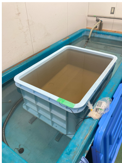
Figure 10: The 400 liter tank for de- veloper. 390 liter developer is inside this tank.
