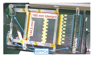
Figure 4: Picture of the new Upstream Charged Veto (UCV) detector. It comprises 0.5 mm thick scintillating fibers to detect charged kaon particles in the beam.
