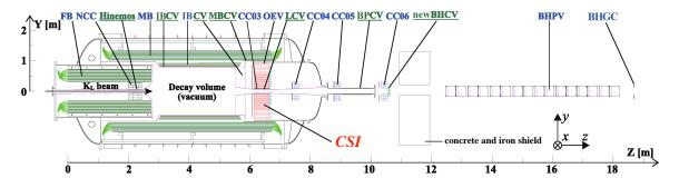
**Figure 1:** Cross sectional view of the KOTO detector. The beam enters from the left into the vacuum decay region. Detector components labeled in blue with their abbreviated names represent photon veto counters, and those labeled in green and underlined represent charged-particle veto counters. CSI is the main CsI calorimeter for detecting photons located at the end of decay region.
