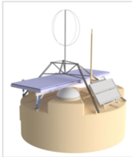
**Figure 5:** Example drawing of a Surface Detector station with AugerPrime components installed.
