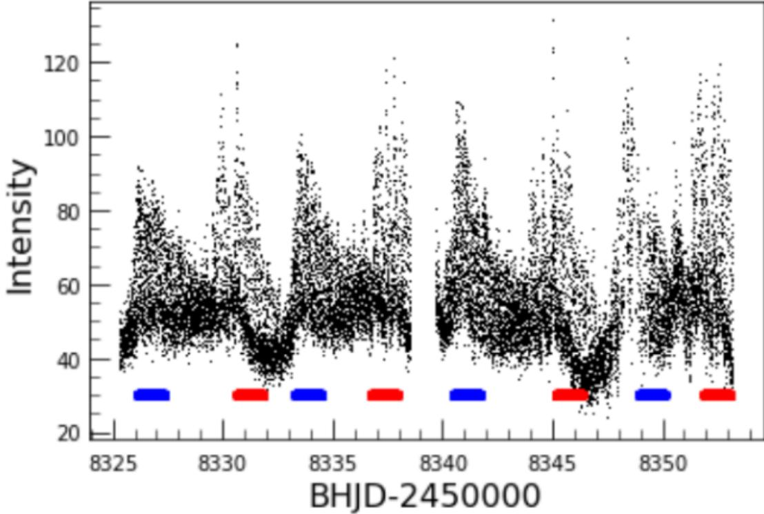
**Figure 1:** The nearly continuous TESS light curve of CD Ind. The time resolution is 2-min and the data span about 28 days. Four beat cycles are clearly seen. While details cannot be resolved on this scale, notice that the individual spin pulses are superimposed on a continuous brightness variation (seen as a dark band) modulated at the beat cycle. The red and blue lines point to data subsets examined in more detail in what follows. Credit: Mason et al. (2020) [8].
