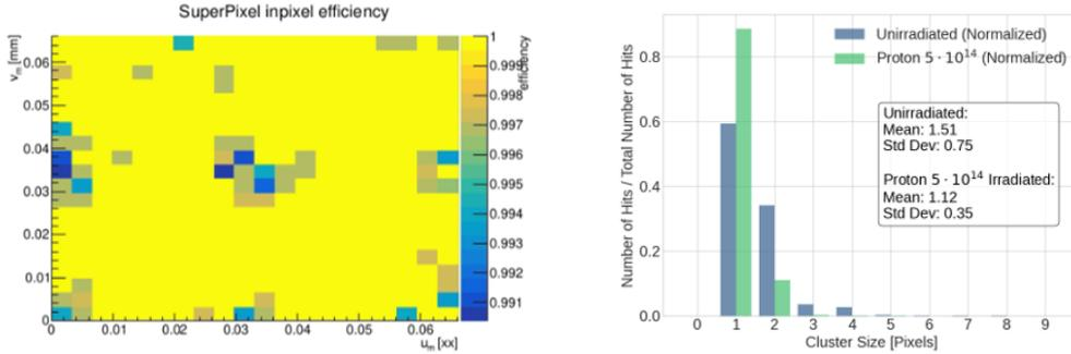
Figure 3,4: Test-beam results for TJ-Monopix2 (threshold at 310  $e^-$  and with irradiated chip W05R16)
