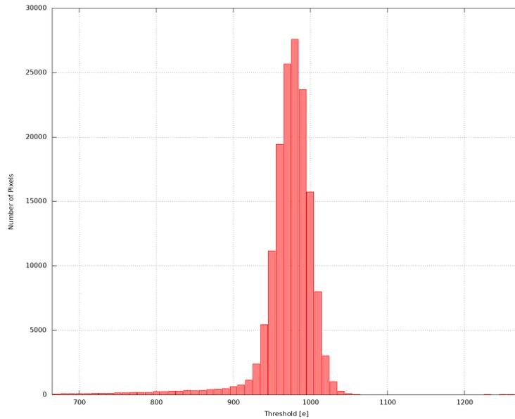
Figure 4 RD53B module thresholds after tuning.
