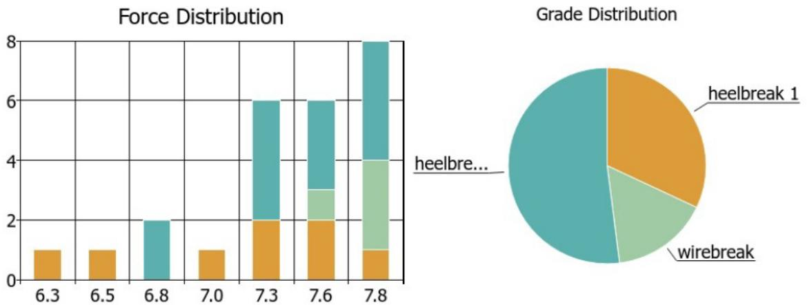
*Figure 2 Pull force distribution in grams obtained for the assembled RD53B module. Heelbreak distribution from flex PCB (heelbreak 1) and from chip (heelbreak 2) sides is also shown.*
