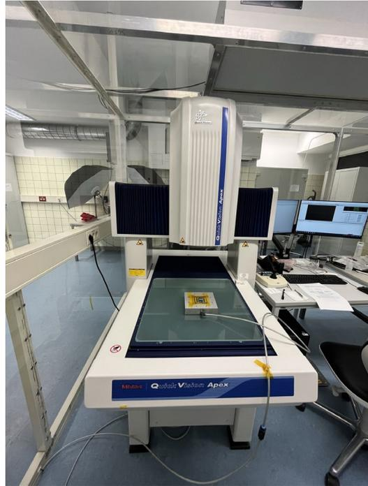
*Figure 1 The Mitutoyo CMM in Siegen with 1.5  $\mu\text{m}$  precision.*
