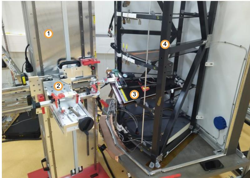
**Figure 5:** Insertion of the first fully loaded pre-production petal in the Endcap System test setup. (1) Insertion tower; (2) Insertion tool; (3) Insertion hand holding the petal (not visible); (4) Endcap System test structure.
