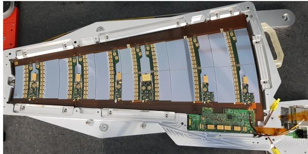
**Figure 3:** A petal fully loaded with six modules, the EoS card and the DCDC boards, mounted at DESY.
