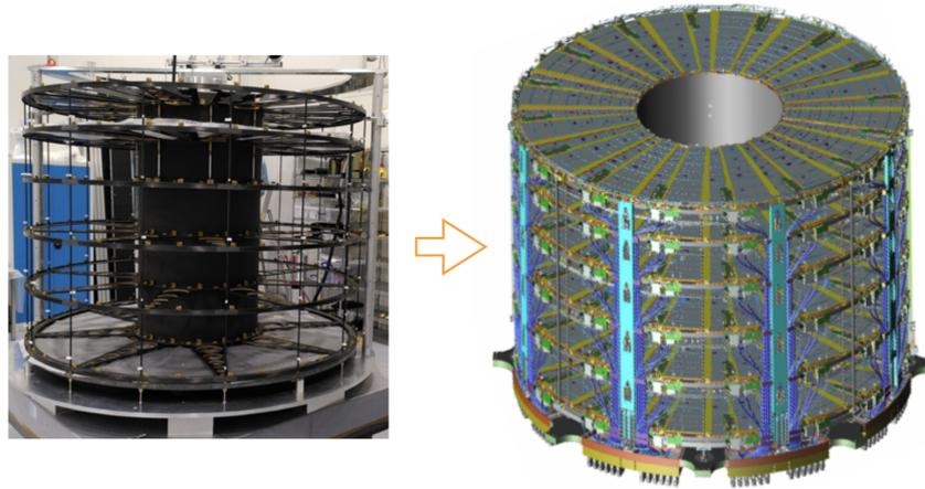
**Figure 2:** *Left:* the empty global mechanical structure of one of the two Endcaps. Photo courtesy of Marcel Vreeswijk (Nikhef). *Right:* CAD design of the final, fully integrated Endcap.
