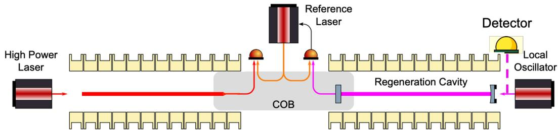
**Figure 2:** Schematic layout of the ALPS II experiment developed for the initial science run.
