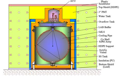
**Figure 2:** A schematic view of the TAO detector and its main components.
