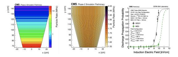
**Figure 4:** Left: Expected background particle rate per HV sector on an ME0 chamber with current eta segmentation. Middle:The middle plot illustrates the anticipated background rate following the implementation of the new redesign. Right: Discharge propagation probability versus the induction electric field for the GE2/1 configuration (black) and ME0 configuration (green) GEM muon detectors [3].
