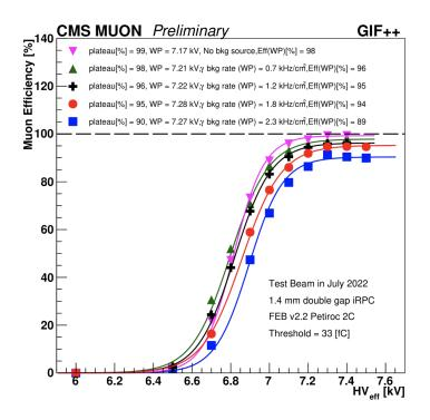
**Figure 2:** Efficiency at working point (WP) measured at 9% with 0.7 kHz/cm<sup>2</sup> (expected Phase II background rate) and 89% at 2.3 kHz/cm<sup>2</sup> (3 times the safe factor for background radiation) [3].
