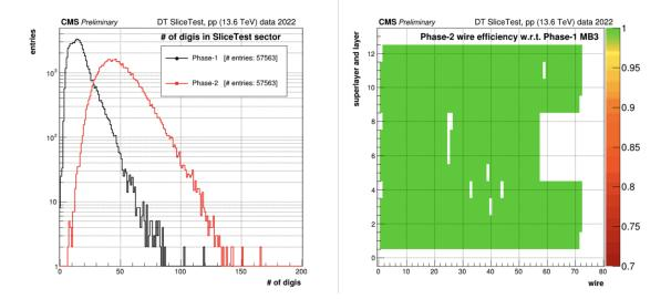
**Figure 1:** Left plot: Distinctive impact of Phase-2's expanded bandwidth: Notice the evident widening of readout windows, 5x broader than legacy. Right plot: the relative efficiency to detect a hit with the Phase-2 readout, when a hit is recorded by the Phase-1 readout in the MB3 station in the slice test [3].
